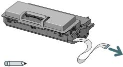
Note: Pull sealing tape completely out of the cartridge.
